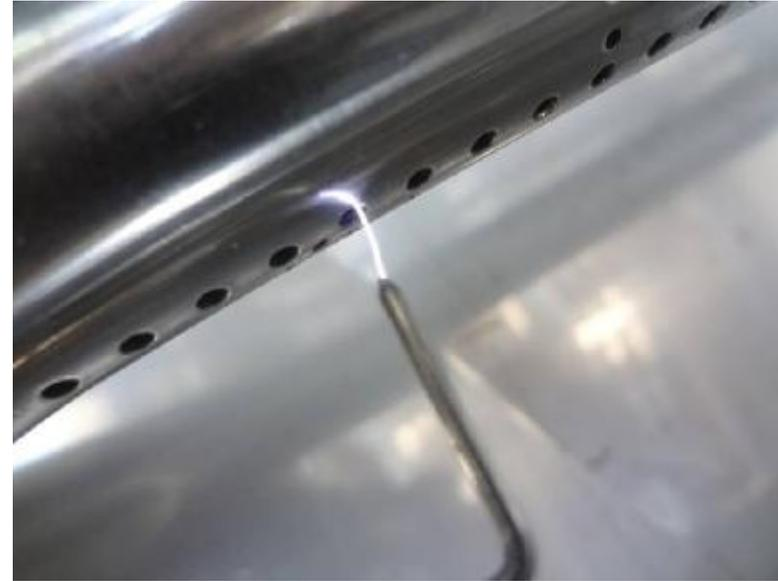
Without the gas on test module by activating the ignition. You should see sparks coming from the electrodes.
