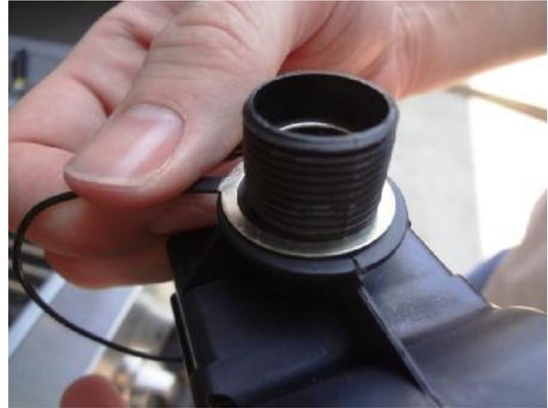
Place the grounding washer at the bottom of the threaded column on the module
