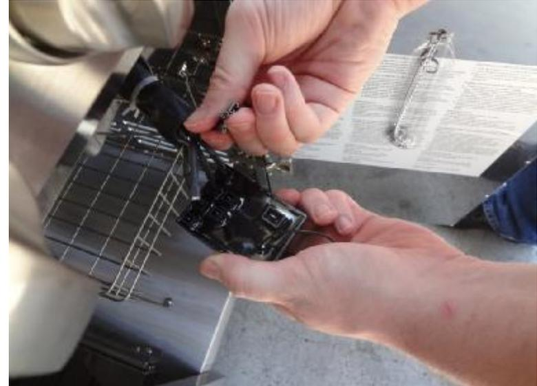
The wires to the ignition electrodes are connected to terminals on the back of the battery box. Loosen the connections by pulling from the base of the wire connection.
