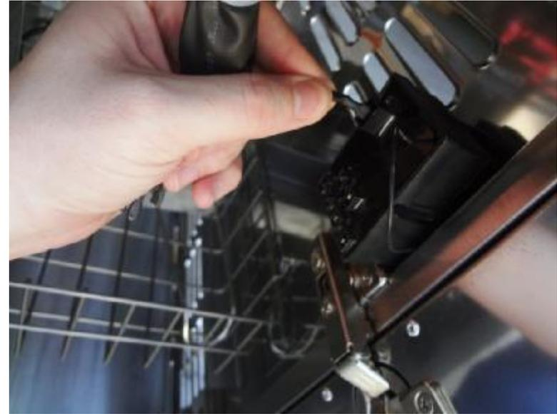
Insert the junction wire first into the larger connection terminal at the back of the new module.
