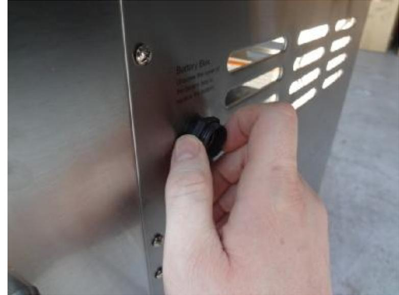
Place the lock washer around the threaded column in the module, making sure the connection is hand tight by turning in a clockwise fashion.
