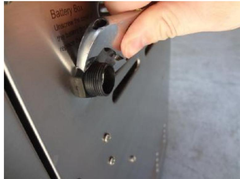
Loosen the lock washer located around the battery by turning it counter-clockwise. You may need a Crescent Wrench to complete this step.
