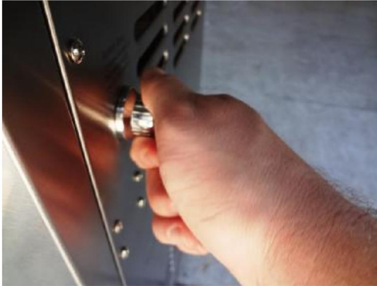
Place the new battery cap onto the module of the unit, turning the cap clockwise to tighten.
