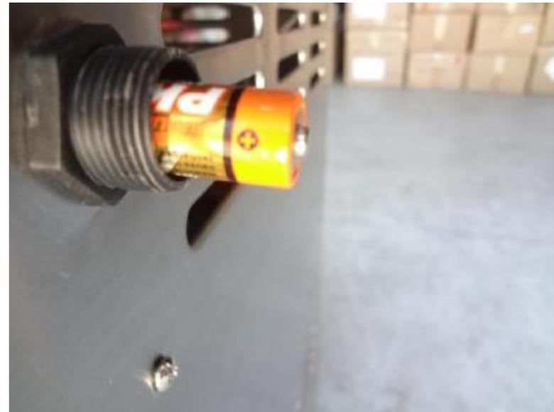
Place the battery into the module with the negative end going in first, and the positive side facing out.
