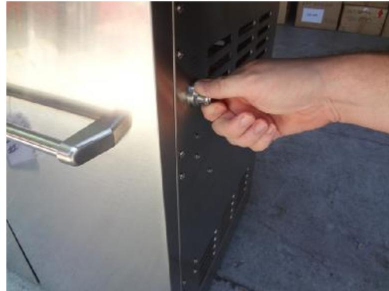
Unscrew the ignition module cap by turning it counter-clockwise.
