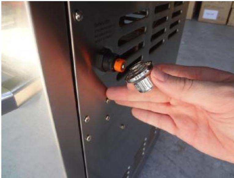
Remove the cap and battery from the ignition module.
