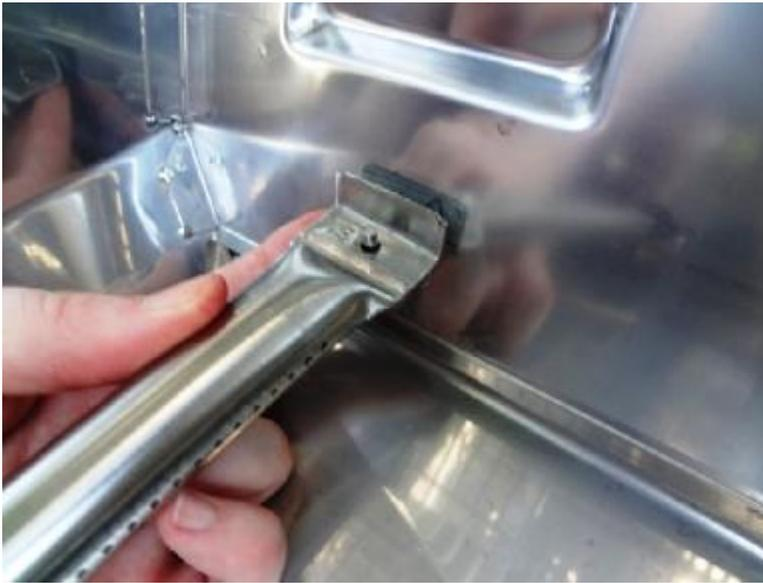
Slide the back end of the burner over the bolt. Do not release your hold on the bolt.
