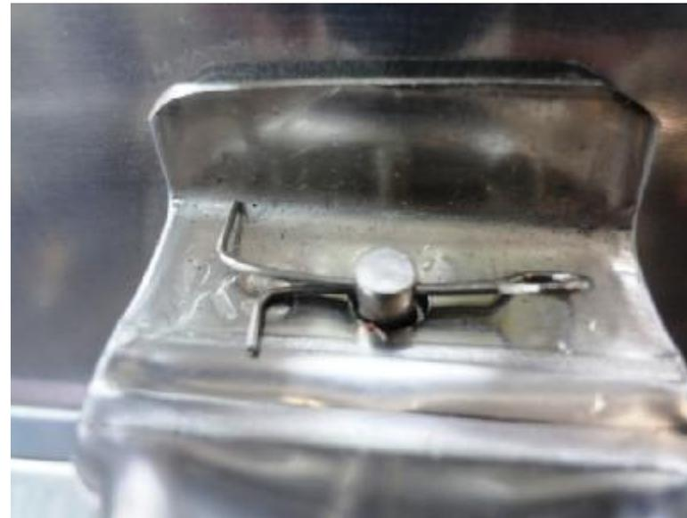
At the end of each burner tube, there will be a connection. In this manual, we will be focusing on the cotter pin assemblies. Other models may have basic screws that are in the same location as the cotter pin assembly
