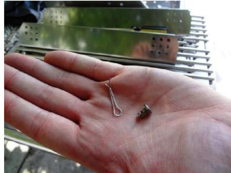
Save the cotter pin, as well as the bolt that the cotter pin mounts through. Set them aside in a safe place as you will be reinstalling those parts on the new burner.
