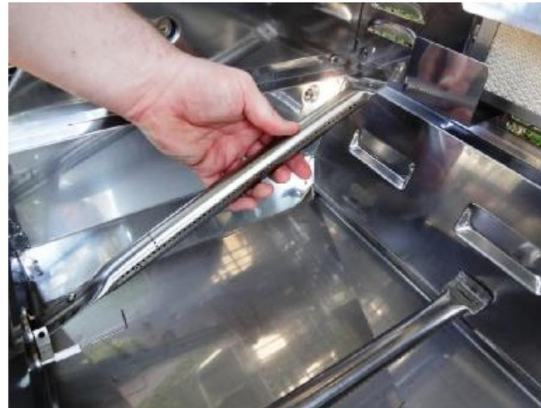
Remove the burner from the bowl assembly by first lifting the end of the burner that mounts to the back of the grill, then pull the rest of the burner from the recess at the front of the bowl assembly
