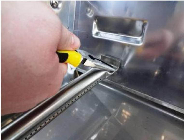
Remove the cotter pin from the bolt. We recommend using needle nosed pliers as you may need to bend the two ends of the cotter pin straight in order to remove it from the bolt.
