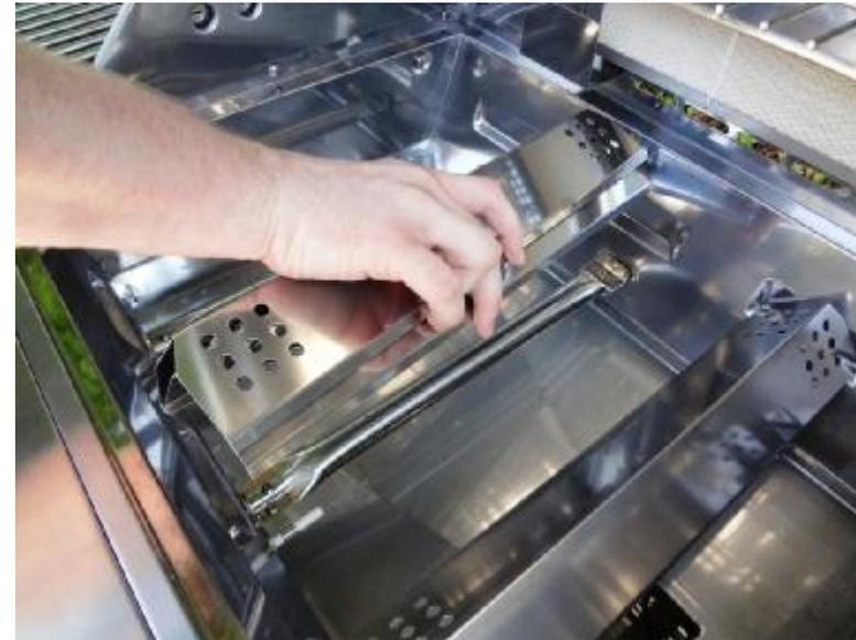
Remove the flame tamers from their original position covering the main burners by lifting the parts up and out of the main bowl assembly. Set the flame tamers aside with the cooking grids.
