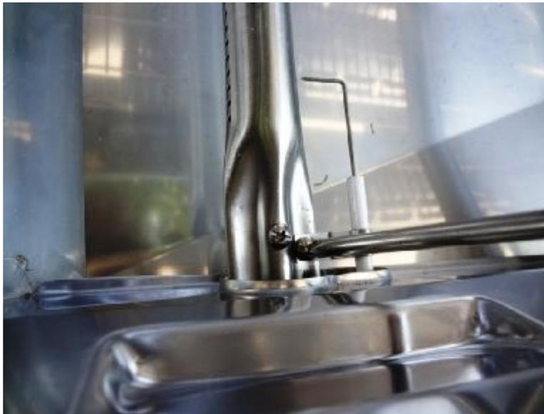
Remove the screw that mounts the ignition electrode to the main burner. The bracket and electrode should be shifted aside slightly as to not be damaged when removing and replacing burner.
