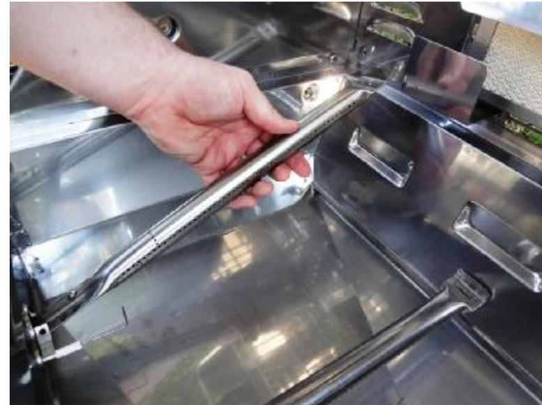
Place the front end of the burner into the recess at the front of the bowl assembly first.
