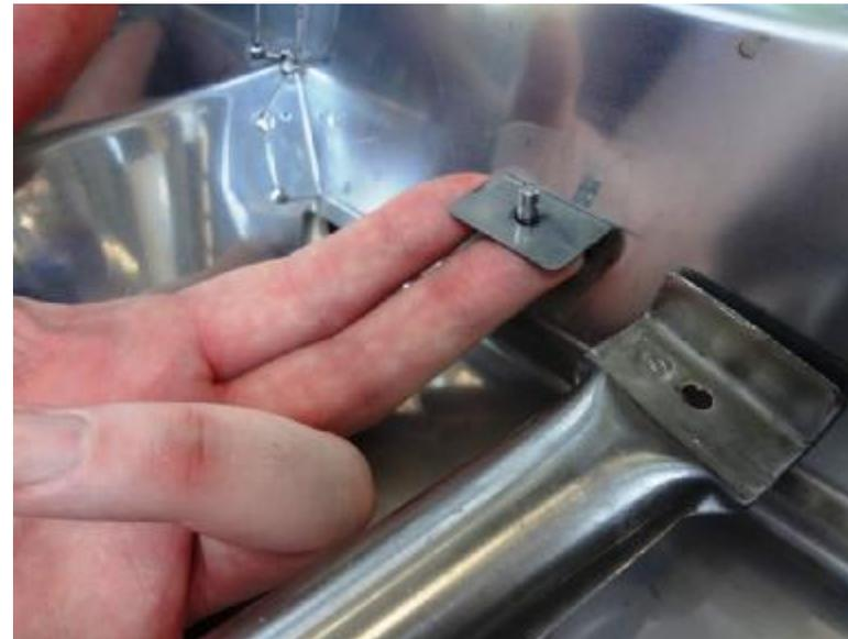
Slide the cotter pin bolt into the bottom of the bracket where the burner mounts. Hold the bolt in place from below.
