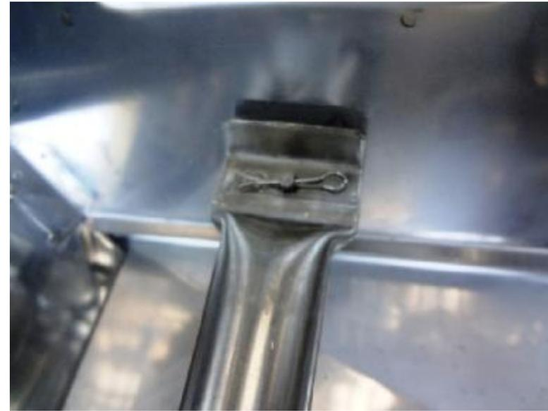
Place the cotter pin through the bolt's end protruding through the top of the burner. You may now release your hold on the bolt as it is held in place by the cotter pin. Bend the end of the cotter pin as to lock the burner in place.
