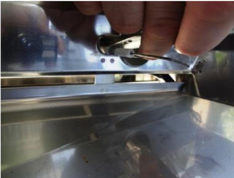
When installing the burner at the front of the unit, make sure that the entrance of the main burner is fitted securely around the valve nozzle where the orifice is located.
