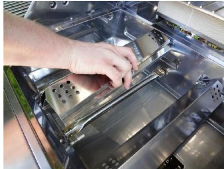
Repeat steps 4 – 15 for each additional burner that needs to be replaced. When you are finished replacing all of the burners, replace the flame tamers over the burners. Set each flame tamer evenly over each of the burners.
