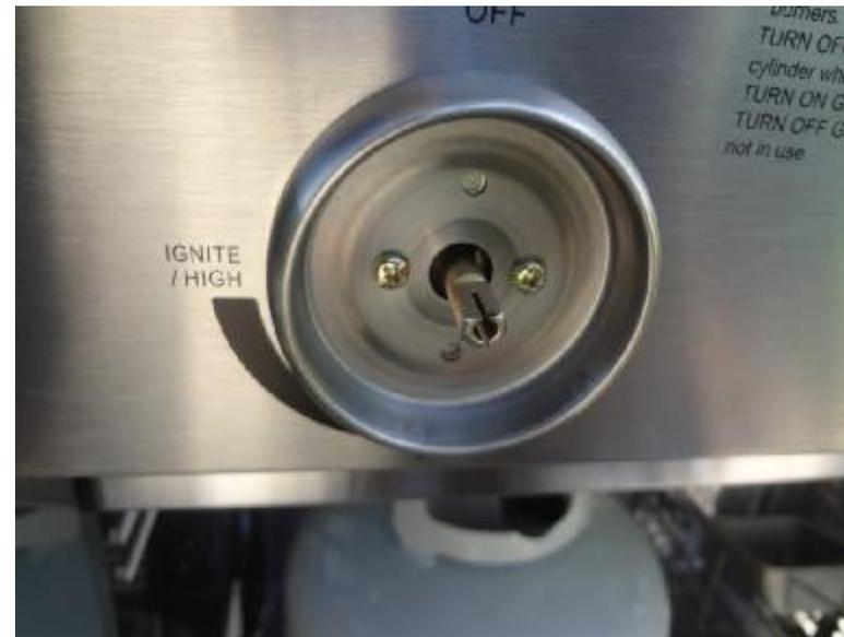
Mount the bezel and the screws to the valve on the front of the control panel centered around the valves stem. Repeat this step with all valves that had been replaced.
