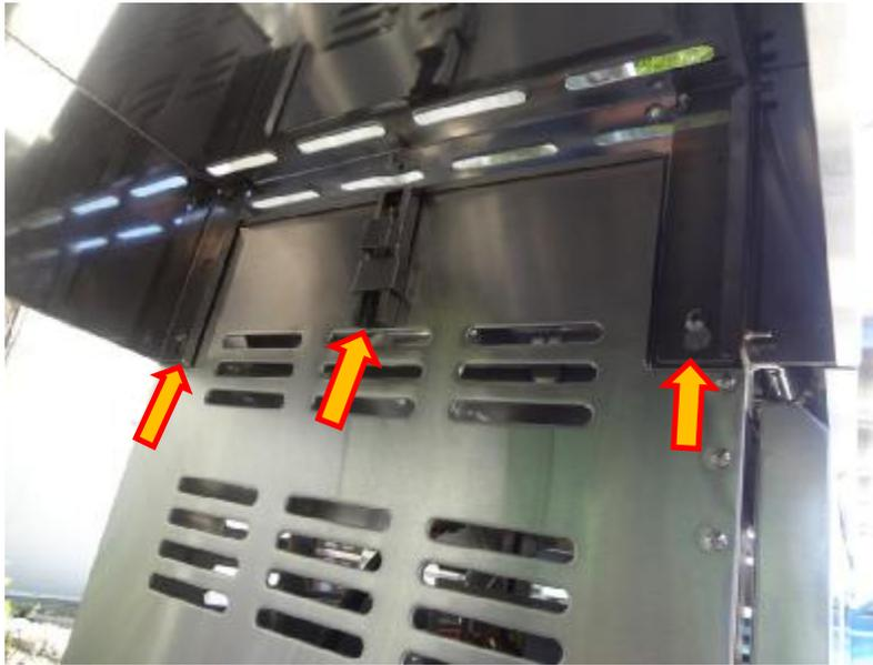
Turn the valve on the propane tank to the off position, and disconnect the gas hose from the propane tank. If the unit has shelves, locate the three screws under the side shelf without the burner. If the grill does not have shelves, skip to Step 10.
