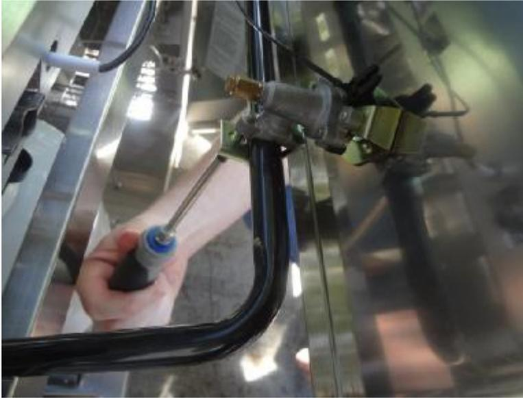
Remove one screw from the bottom of the valve where the manifold retainer bracket clamps the valve to the manifold. Repeat this step for each of the valves on the main control panel where valves need to be replaced.
