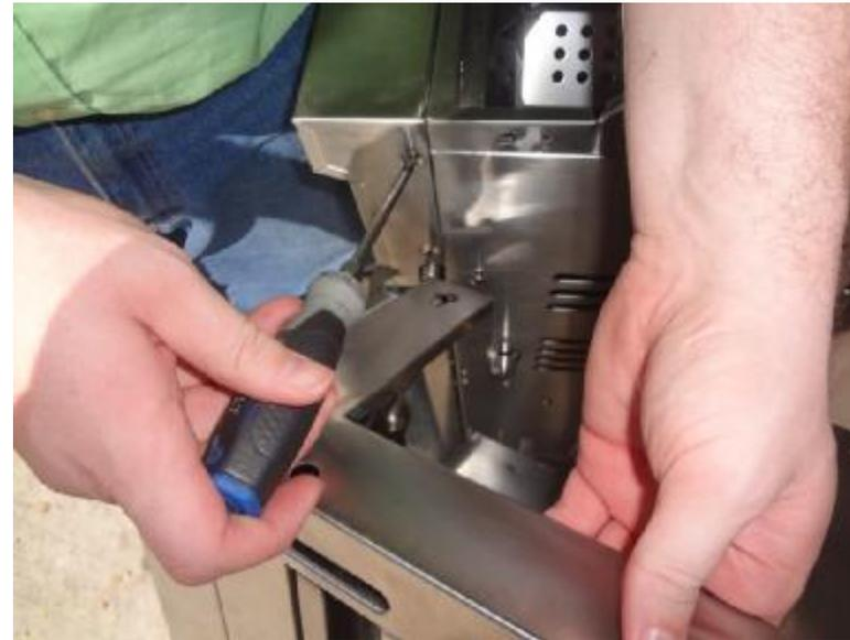
Remove the screws from the side of the control panel where the gas flex line extends towards the shelf with a side burner. Be careful not to kink or otherwise damage the flex line.
