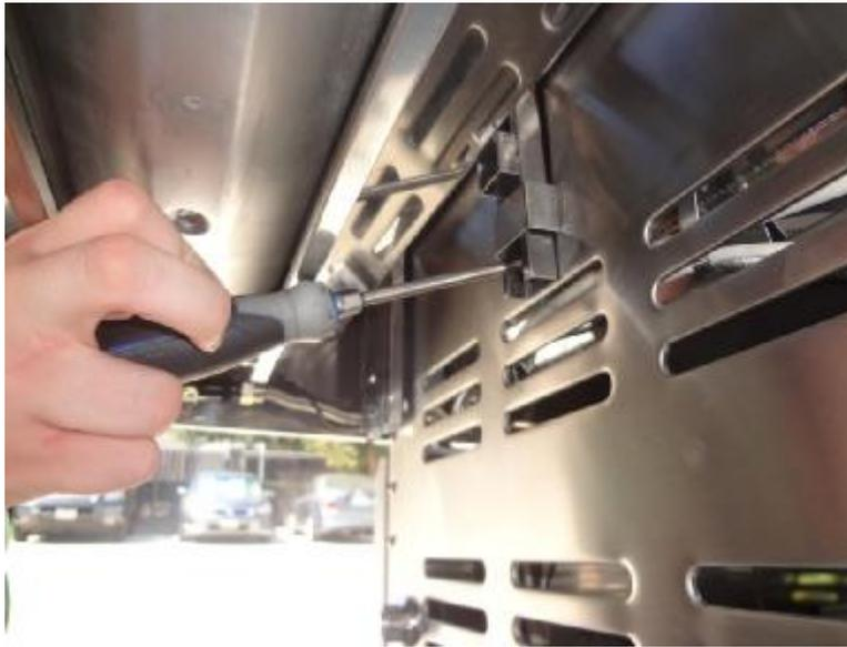
Secure the screw that goes into the center post of the side shelf, and then tighten the screws that mount on the left and right via the keyhole slots. Using the same method install the opposing side shelf.
