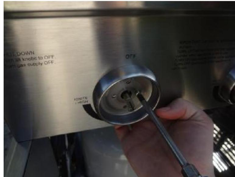
Remove the two screws from the bezel on the left and right side of the valve stem protruding from the center. Repeat this step for each of the bezels on the main control panel where valves need to be replaced.
