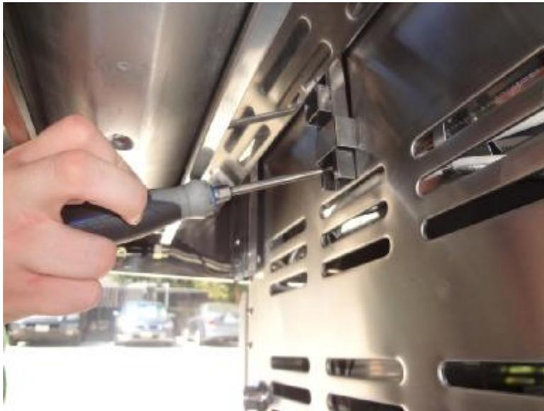
Secure the screw that goes into the center post of the side shelf, and then tighten the screws that mount on the left and right via the keyhole slots. Using the same method install the opposing side shelf.
