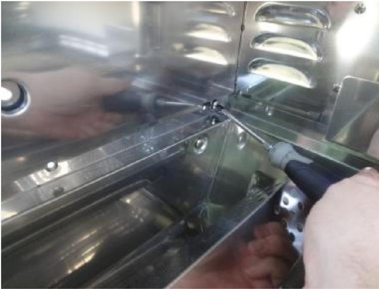
Remove the screws that connect the side shelf to the main body of the grill.
