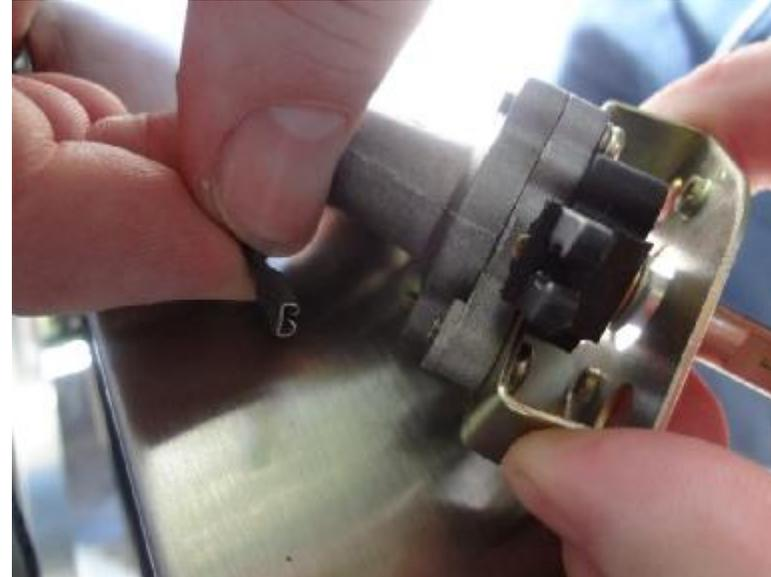
Replace the junction wire connection from the previous valve onto the replacement valve. The wire mounts above the main body of the valve.
