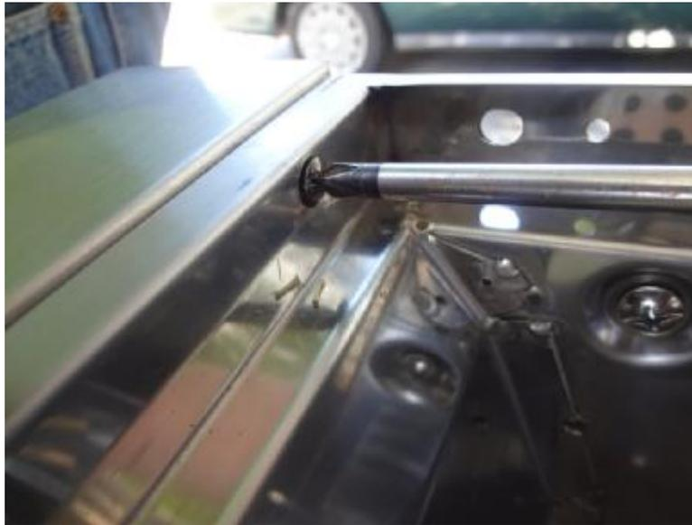
Remove the screws from inside the holes located along the inside lip of the grill, where grill sits.
