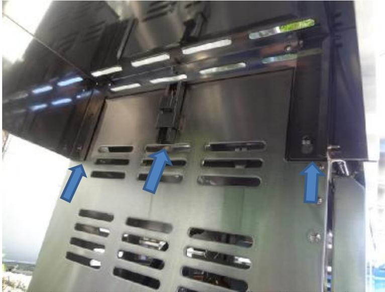
Turn the valve on the propane tank to the off position, and disconnect the gas hose from the propane tank. If the unit has shelves, locate the three screws under the side shelf without the burner. If the grill has no shelves, move to step 10.”
