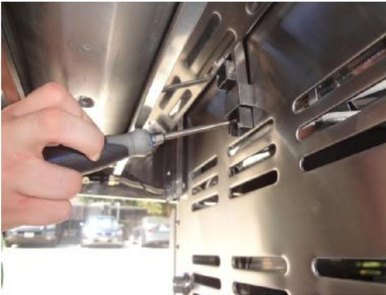
Repeat steps 1-5 with the side shelf containing the burner. Some models do not have a burner in either side so simply remove both side shelves as normal.
