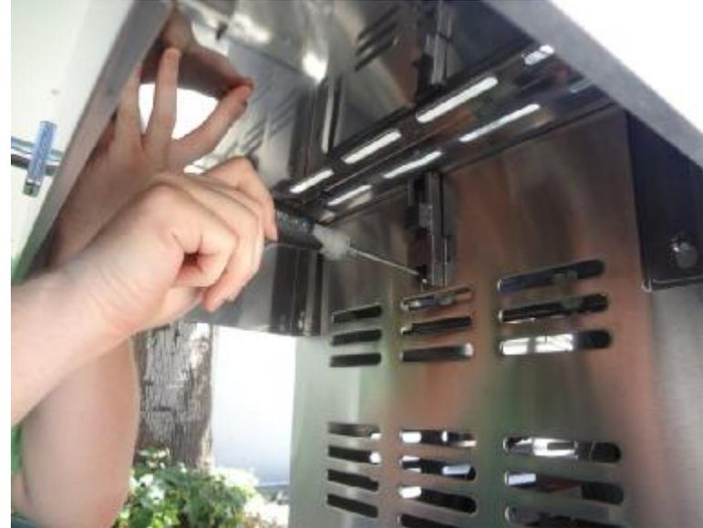
Remove the screw on the center post and loosen the screws on the left and right posts.
