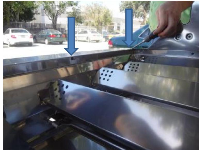
Locate the holes on the inside of the bowl assembly along the lip where the cooking grids sit in place.
