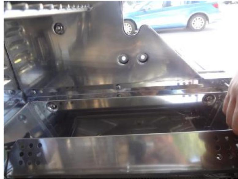
Mount the side shelf to one side of the unit, securing the units with the keyhole slots to the screw heads still mounted onto the body of the grill. Reinstall the three screws to the side shelf from the inside of the unit.
