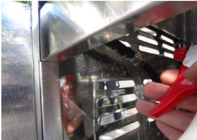
Connect the gas hose to the propane tank. Coat the entire length of the gas hose, including the coupling nuts on both ends, with the soapy water solution. Also apply the soapy water solution to the gas valves you just replaced.
