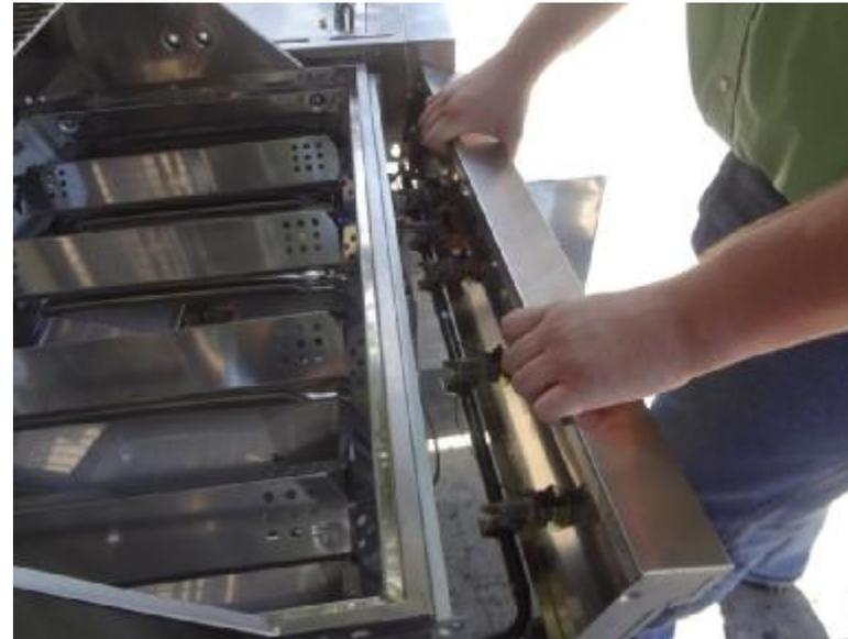
Free the control panel from the main body of the grill. There are still going to be component parts of the grill that are connected to the control panel, so take extra care with this step to avoid damaging those components.
