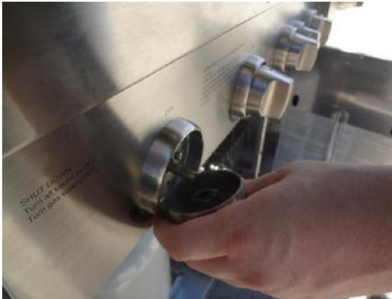
Reconnect the burner knob to the valve stem. Secure the screw if necessary by using an Allen key. Repeat this step for all valves that have been replaced.
