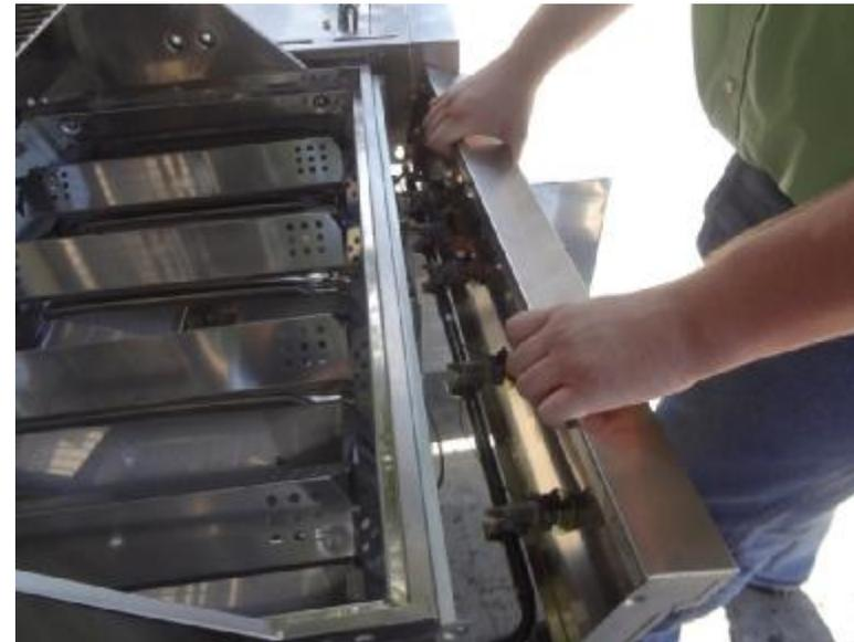
Replace control panel to the front of the grill body, making sure the valve nozzles are aligned properly into the burners.
