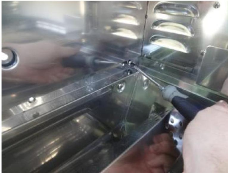
Remove the screws that connect the side shelf to the main body of the grill.
