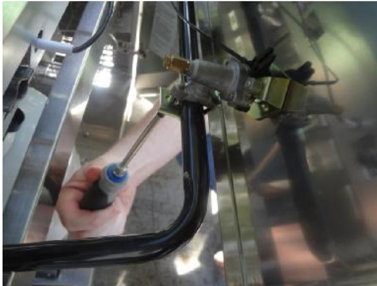
Install the replacement valve onto the manifold, placing the valve stem through the hole in the control panel. Hook the manifold retainer bracket to the manifold and tighten the screw to secure the bracket. Repeat steps 16 – 21 for each valve that needs to be replaced.
