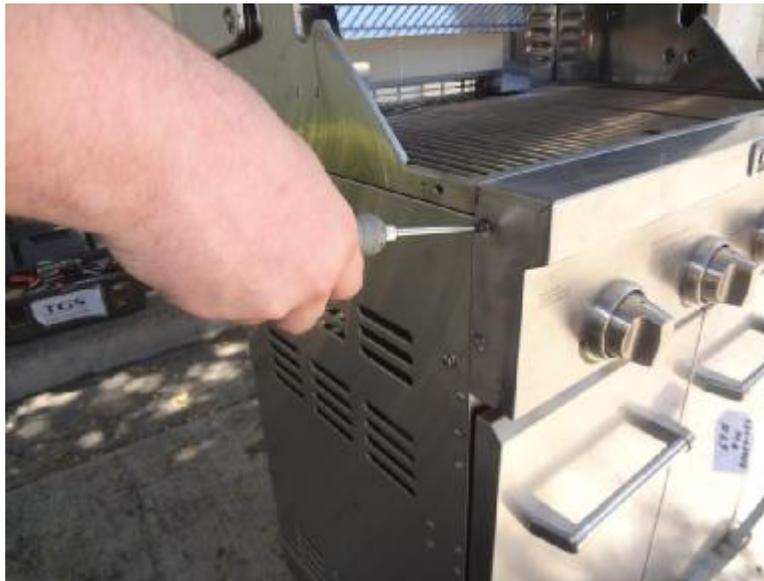
Remove the screws from the side of the control panel where you removed the shelf without a burner.
