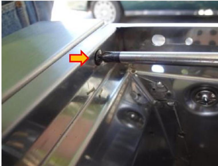
Remove the screws from inside the holes located along the inside lip of the grill, where grill sits.
