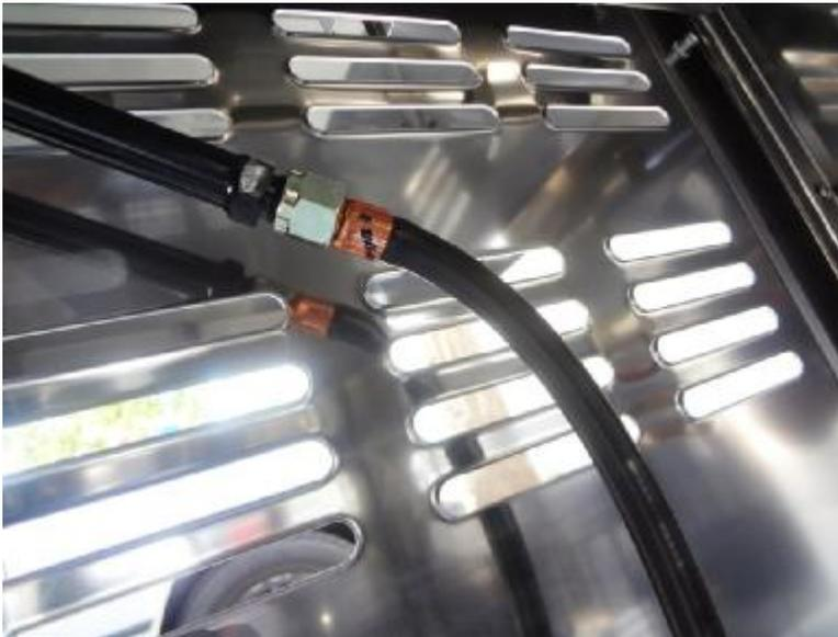
Locate the opposite end of the regulators gas hose where the brass fitting connects to the manifold.
