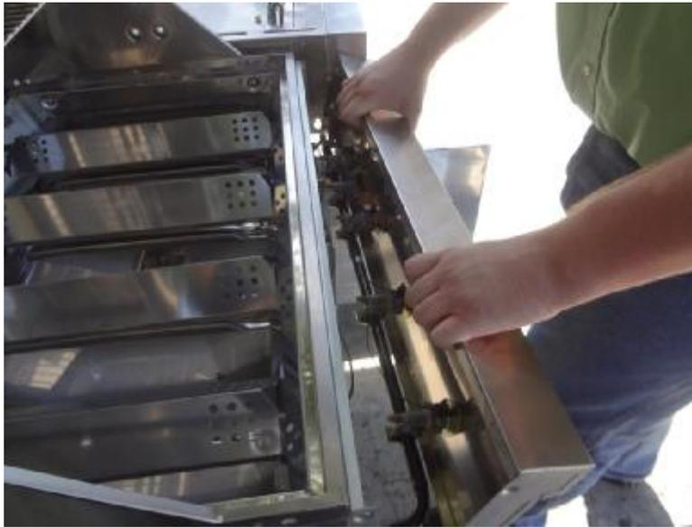
Replace control panel to the front of the grill body, making sure the valve nozzles are aligned properly into the burners.
