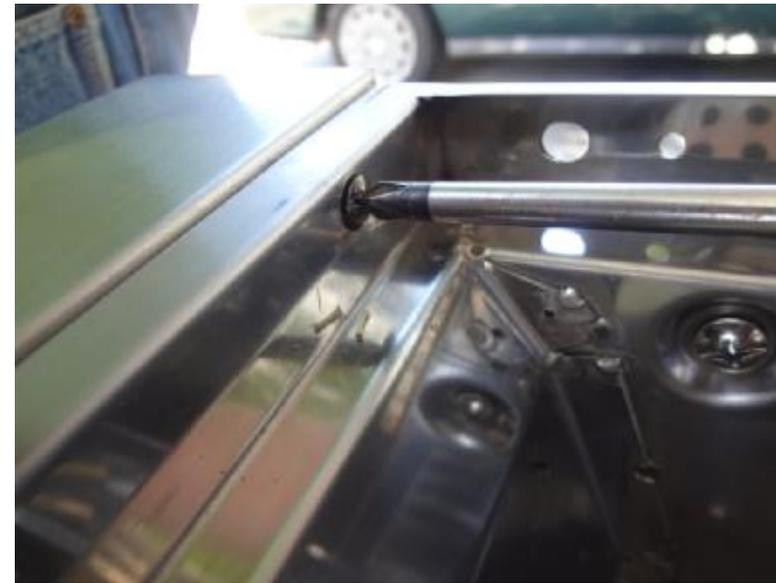
Re-install the screws on the inside lip of the main bowl area where the cooking grids set into. These screws will help support and secure the control panel.
