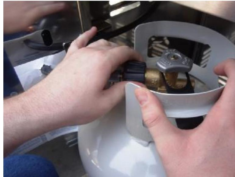
Place the propane tank into the opening in the propane tank compartment and re-attach the regulator coupling nut to the propane tank by turning it clockwise.
