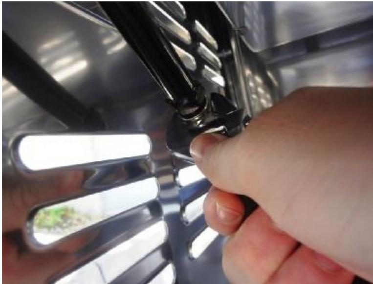
Using the two wrenches, tighten the brass fitting onto the manifold. Do not over-tighten the connection.
