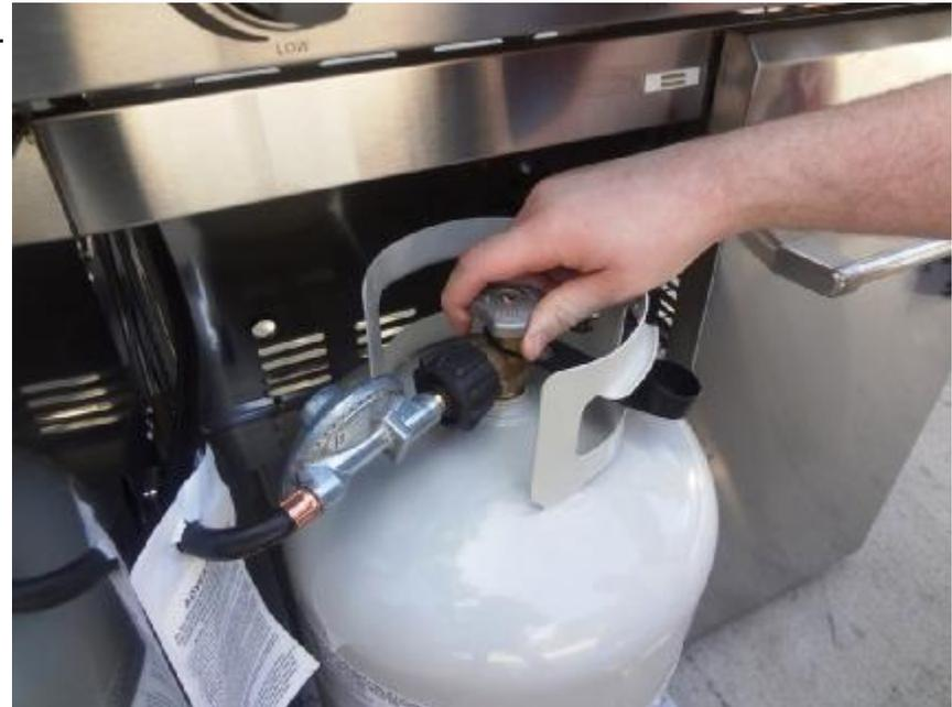
Turn the propane tank gas valve clockwise to the off position.
