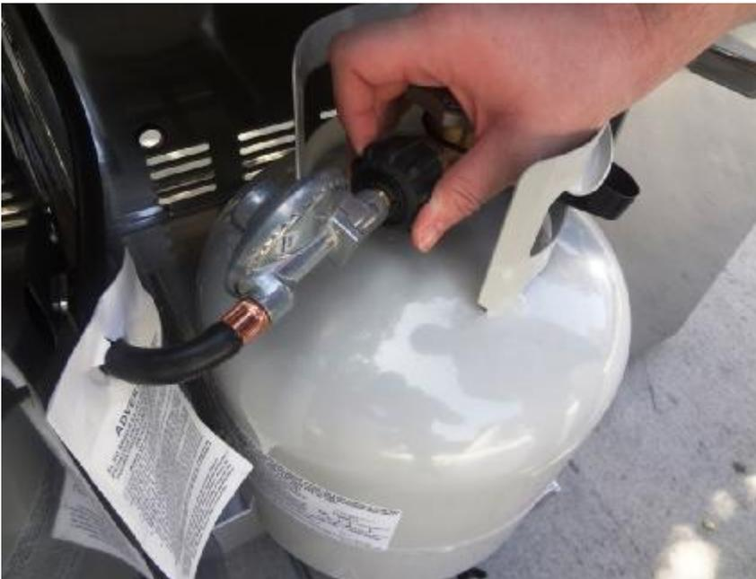
Remove the regulator coupling nut from the propane tank by turning the coupling nut counter-clockwise.
