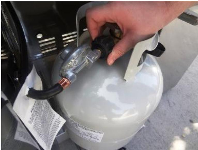
Remove the regulator coupling nut from the propane tank by turning the coupling nut counter-clockwise.
