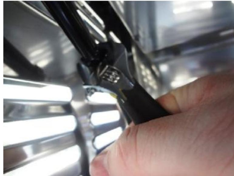
Using an adjustable wrench, disconnect the brass fitting by turning it counter-clockwise. Secure the manifold using another wrench, while disconnecting the brass fitting.
