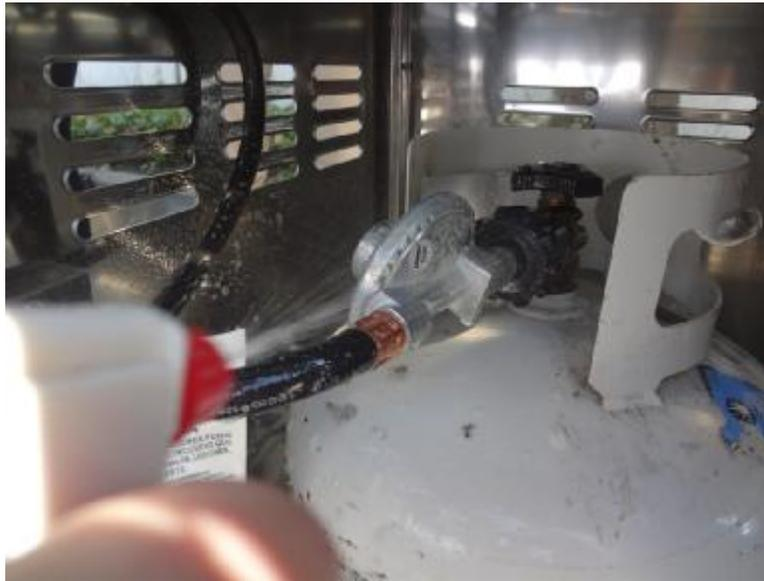
Apply the soapy water solution to the regulator, coupling nut, gas hose, and the connection to the manifold. Make sure to coat the entire length and both ends of the gas hose.”
