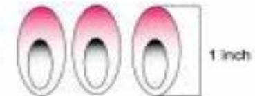
With the valves in place, there should be a 1-inch flame on the burners while the unit is in operation at the high setting. The grill should reach temperatures in excess of 500 degrees within 10 – 15 minutes.
