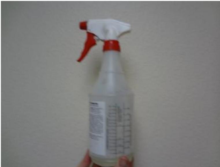
Prepare a 50/50 solution made of water and ammonia-free dish detergent. Prepare the soapy water solution to be applied to parts using either a spray bottle or a brush.
