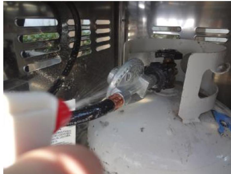
Apply ammonia-free soapy water solution to the regulator hose, and relevant connections using your chosen application method.
