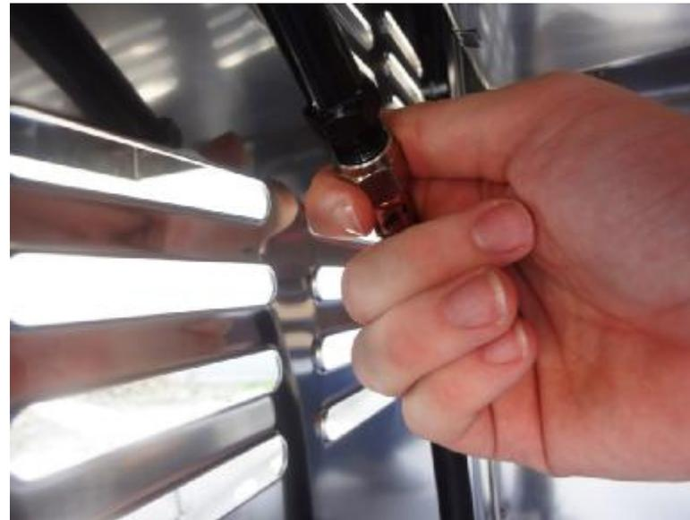
Attach the new regulator gas hose by turning the brass fitting clockwise onto the manifold until it is hand-tight.
