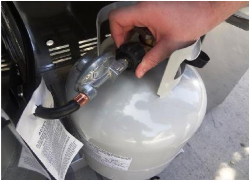
Re-attach the regulator coupling nut to the propane tank by turning it clockwise. Open the propane tank gas valve by turning it counter-clockwise until it will no longer turn.
