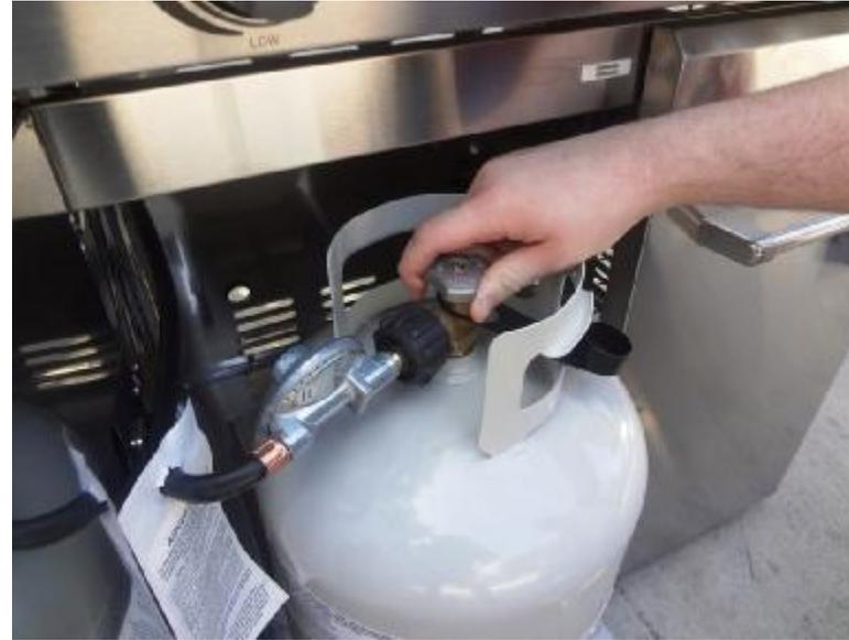
Open the propane tank gas valve by turning it counter-clockwise until it will no longer turn.
