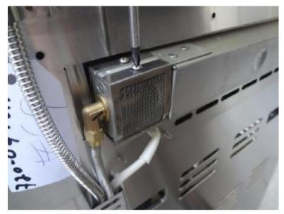
Replace the spider guard mesh screen back into position and reinstall the screw into the top to secure the mesh guard.
