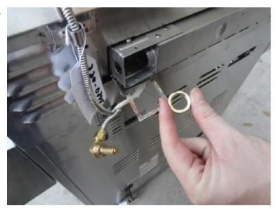
Remove the brass ring from the brass elbow, and pull the elbow from the hole where it is mounted to free the rotisserie burner.
