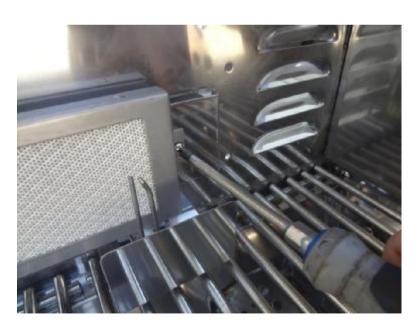
Reinstall the screw into the bracket of the rotisserie burner.
