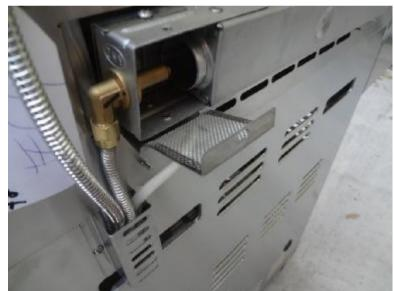
Carefully open the spider mesh guard screen over the rotisserie burner orifice once the screw has been removed.
