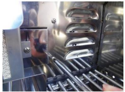
Remove the two screws to the right side of the rotisserie burner.
