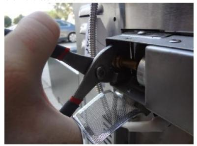
Using a wrench or pliers, turn the brass ring that mounts the brass elbow to the orifice of the grill.
