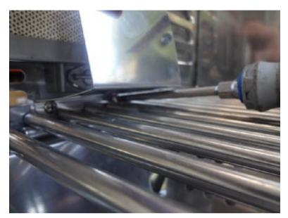
Remove the rotisserie burner gas collector from both the right and left sides of the unit. They mount by using two screws on the bottom of the unit. You may need to remove the grilling grates.
