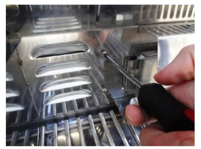
Install the screws to the rear baffle on the left side by installing the screws from the inside of the bowl assembly as shown.
