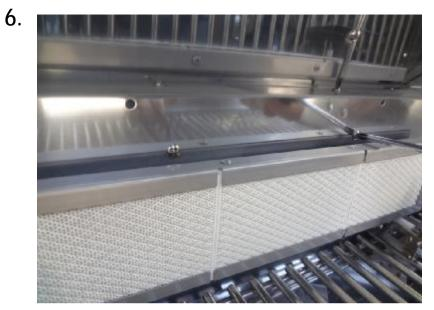
Remove the two screws to the top of the burner. They correspond with the rear baffle on the back of the unit. Be prepared to support the baffle as they are the last screws.
