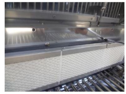
Reinstall the screws that mount the rear baffle at the top by installing screws from the inside of the bowl assembly as shown.
