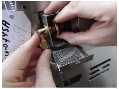
Mount the Rotisserie Brass Elbow into the burner and tighten the brass nut onto the thread. Tighten this nut with wrench to ensure the brass elbow is secure.
