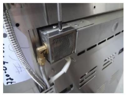
Go to the back of the unit and remove a single screw from the top of the bracket that secures the spider guard mesh screen over the rotisserie burner orifice.
