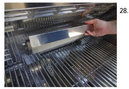
Reinstall the rotisserie burner heat shield. You will need a second set of hands to hold the heat shield in place while the screws are reinstalled on the back of the unit.
