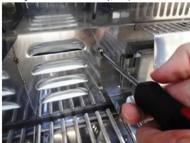
Remove the two screws to the left side of the rotisserie burner.
