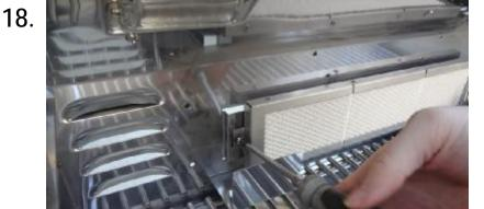
Install the left screw into the bracket of the rotisserie burner as it was previously.
