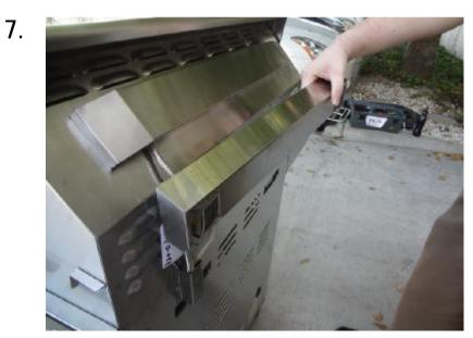
Remove the rear baffle now that the screws have been taken out. Set the part in a safe dry place.
