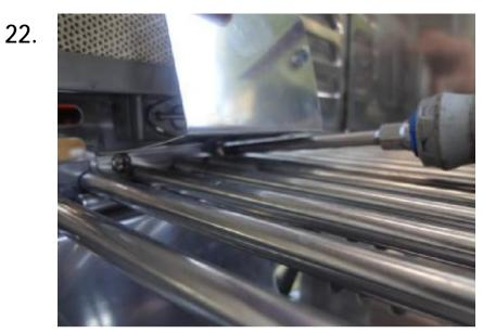
Reinstall the rotisserie burner gas collector. Two screws mount the bracket from the bottom.
