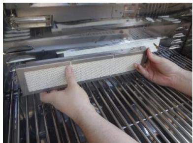
Free the old Rotisserie burner from the unit by sliding the unit to the left slightly and then pulling the unit forward until it is freed.
