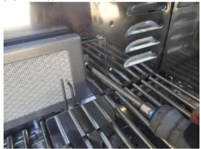
Remove the right screw of the rotisserie burner bracket that mounts the burner to the back of the unit.
