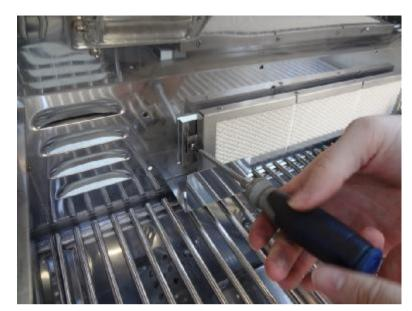
Remove the left screw of the rotisserie burner bracket that mounts the burner to the back of the unit.
