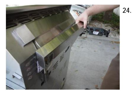
Reinstall the rear baffle on the back of the unit. You may need a second set of hands to hold the baffle in place while the screws are installed during the next step.
