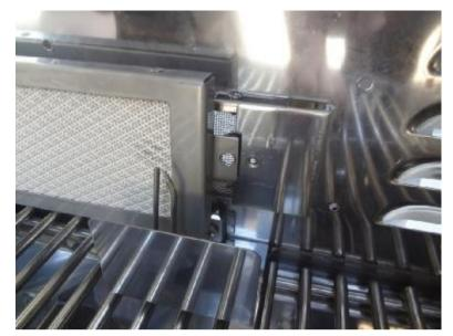
Slide the new rotisserie burner into place, aligning the burner into the bracket, over the hole as pictured in Step 8.
