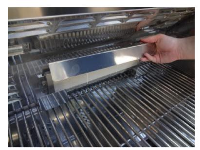
Remove the rotisserie burner heat shield from the unit now that the screws are removed. Set the part in a safe dry place.
