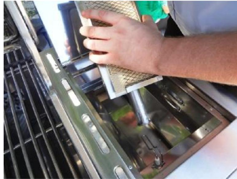
Remove the sear burner from the bowl assembly. Lift from the back end of the unit first.
