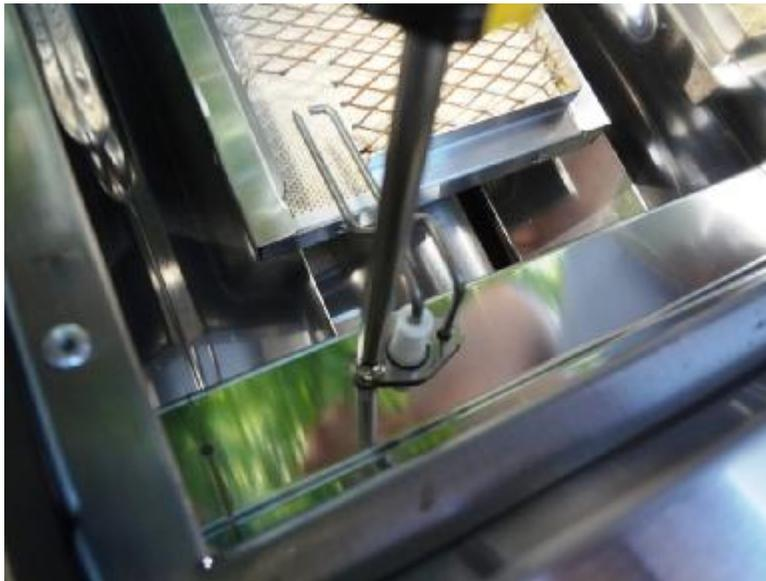
Install the screw to the ignition electrode removed on step 2. Make sure that the ignition is placed over the searing side burner near the opening in the grate of the burner.
