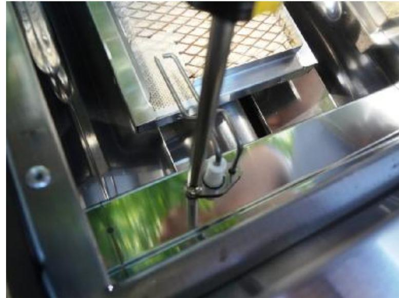
The ignition electrode mounts by one or two screws. Remove and save these screws.
