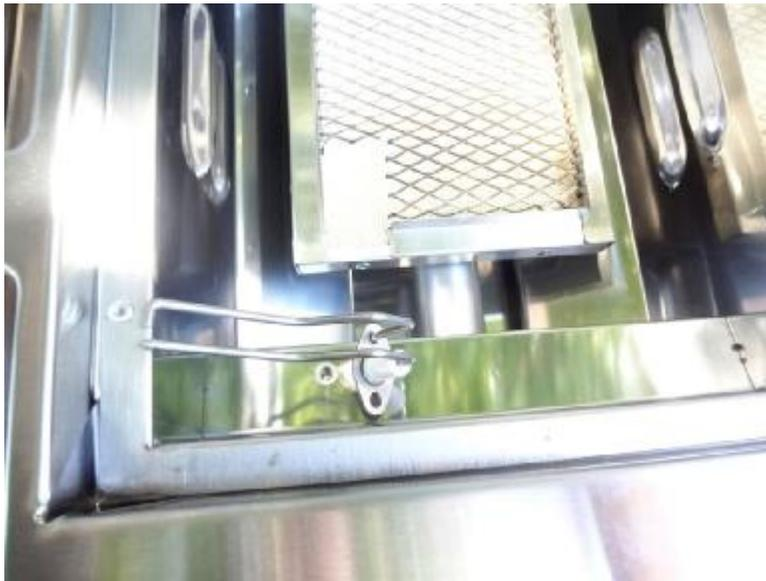
Now that the ignition electrodes are free, turn the part to the side so it will not interfere with the removal of your sear burner.
