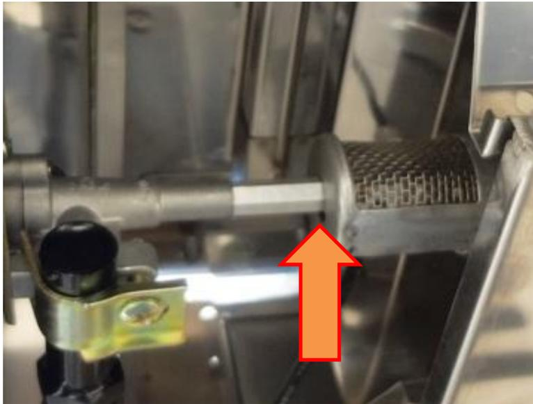
Check that the valve nozzle is inserted into and directing the flow of gas into the sear burner, and that the connection is secure. This is best done by looking from the underside of the unit.
