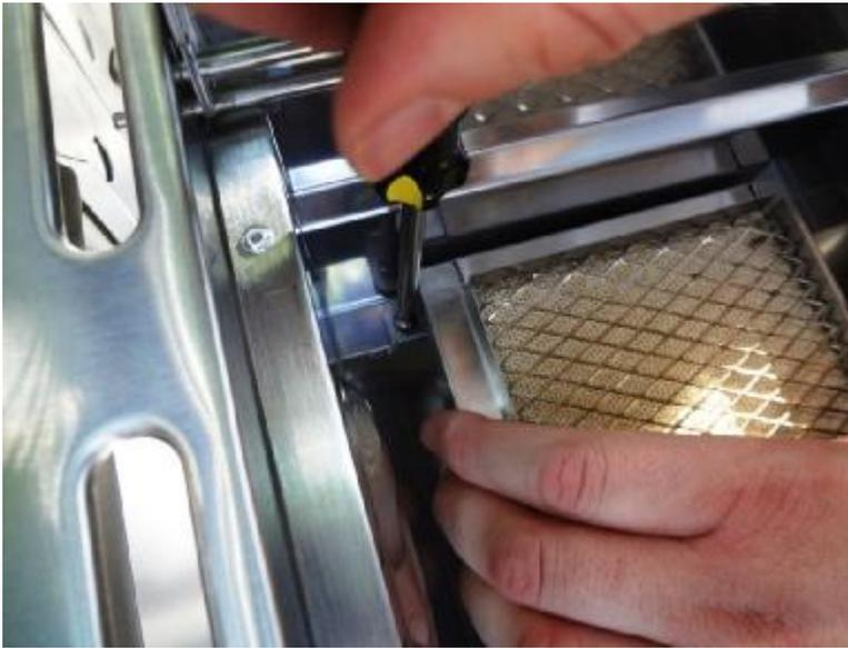
Remove the screws that mount the sear burner to the back of the grill. Save these screws as they will be required to install the new unit.
