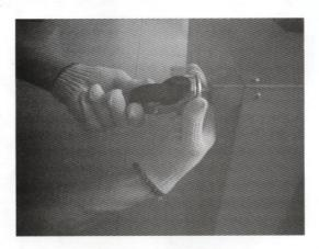
b. The handles have the necessary screws already inserted in the handles. Unscrew these screws, line up the handle with the holes on the side of top lid, insert the screws from the inside of the lid, and firmly tighten the screws.
