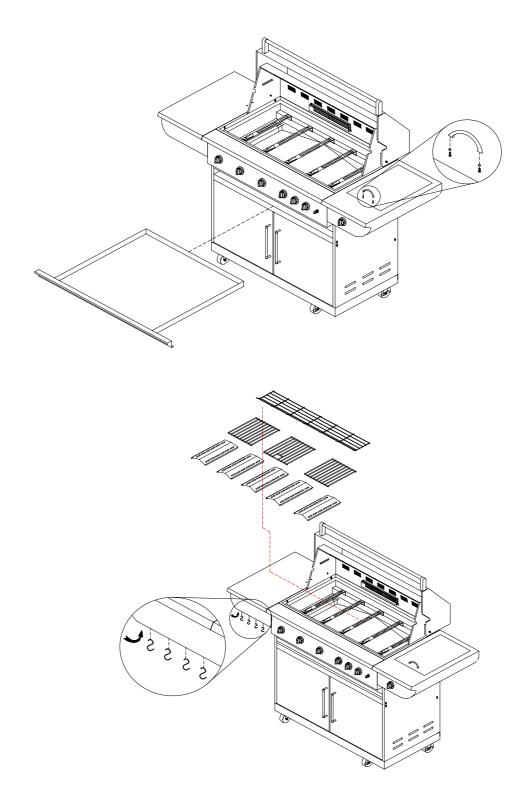
♦ 2 pieces of 1/4"x10mm screw and 2 pieces of 1/4"split lock for rotisserie mount are already screwed into the right side panel of the grill. Remove the screws and install the rotisserie motor mount as shown in the figure below. Assemble the rotisserie skewer as shown in the figure below.
