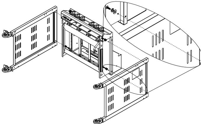
**STEP 3B:** Assemble bottom panel to side panels with 4-1/4 x 1 1/2" screws.
