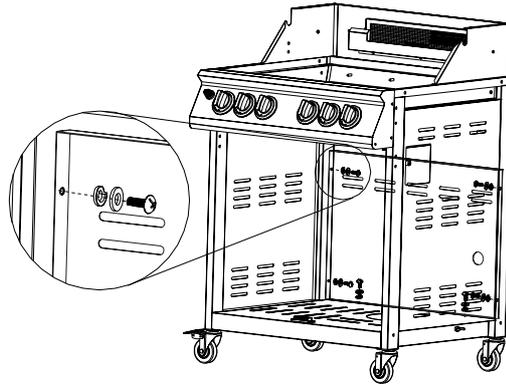
**STEP 5A:** Insert both doors' hinge pins through the holes on the bottom of the bottom panel. Make sure the washers are in place.
