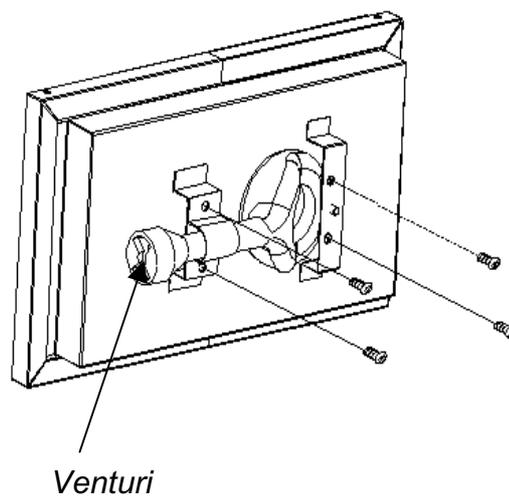
Step 9: Insert valve stem assembly into burner into venturi
