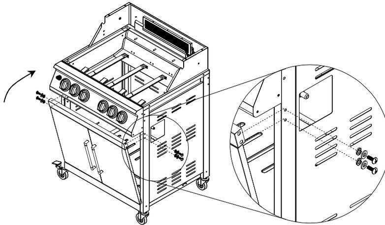
**STEP 5C:** Install the lid back in place using the same hardware kept from step 2.
