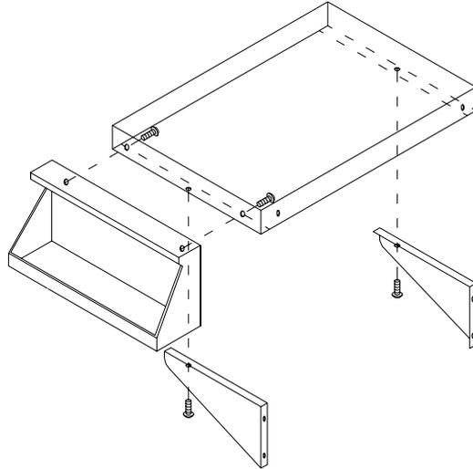
**STEP 6B:** Use two screws and lock washers to fasten the control panel to the side shelf. Do not tighten these screws until the valve stem protrudes through the control panel (step 8). Use two screws and lock washes to fasten the support brackets to the side burner as illustrated.
