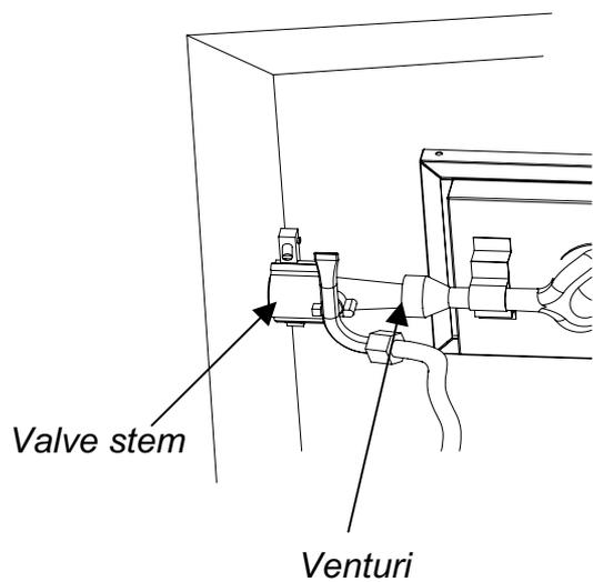
Step 10: Insert valve stem assembly face-plate.
