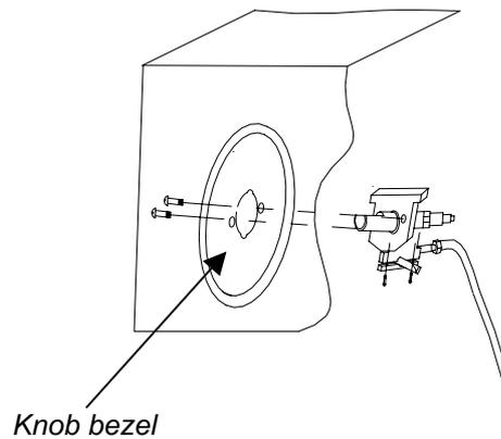
Step 13; Tighten all 4(four) screws on the "U" brackets on the burner, then connect the ignition wire on to valve.
