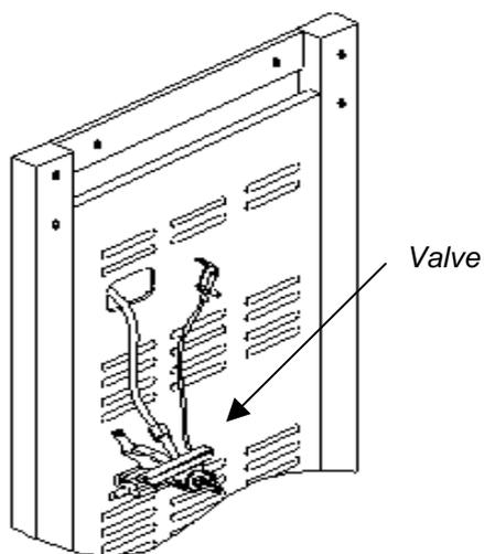
Step 8: Remove 4(four) screws & washers from the "U" brackets on the side burner
