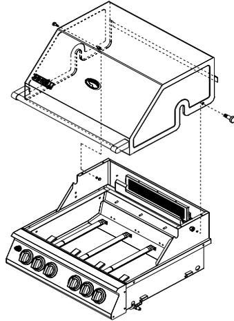
**STEP 3A:** Tip back the grill head have it lay on the floor. Line up and assemble the right & left side panels & secure with 4 1/4"x 20x1 1/2" screws from the four inside corners of the grill housing.
