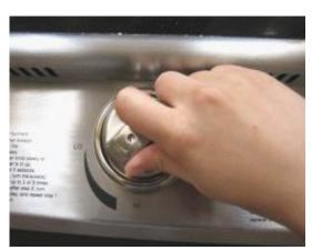
Step 2. Push and turn one of main or side burner knobs to HI position
